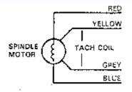
Motor coil = 17 ohms Tach coil = 175 ohms at rest Tach coil = 135 - 190 ohms in motion
