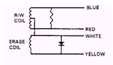
R/W end to end = 32.4 ohms R/w end to centertap = 16.3 ohms Erase coil end to end
