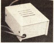
It weighs only 2.5 lbs. and features an input of 105-125 VAC at 60 HZ and 43 Watts at full load. A .5 AMP Primary Fuse and 2 conductor with ground line cord is part of this package.
