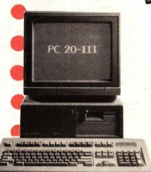
COMMODORE PC 20-III Includes all the exclusive features of the Commodore PC 10-III but also includes a standard 20MB hard disk that does not use an expansion slot. It still leaves room for 2 more half-height storage devices. The PC 20-III includes a built-in RS232C serial port as well as a Centronics parallel port and even a mouse port. And the 3 full length IBM PC/XT compatible slots allow for maximum expandability which make it ideally suited for your business environment.
