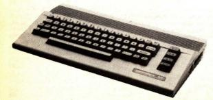
THE 64C COMPUTER. The 64C resembles the sloped design of the C128 computer. It includes all the key features of the C64 including 64K RAM, 20K ROM, 3-voice sound capability, 16 colors and 320x200 resolution graphics. Uses the same hardware and software packages as C64
