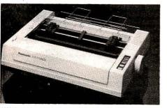
KX-P10801. Dot matrix, NLQ at 24 cps and draft speed of 120 cps. 9 wire print head and a life of 100 million characters, parallel interface, tractor and friction feed. Two year warranty. Sug. Retail \$269.95 A27851 Panasonic KX-1080i \$189.95
